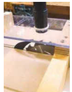
PIC 6. Cross-cut sled in place showing extraction and safety block on the rear
